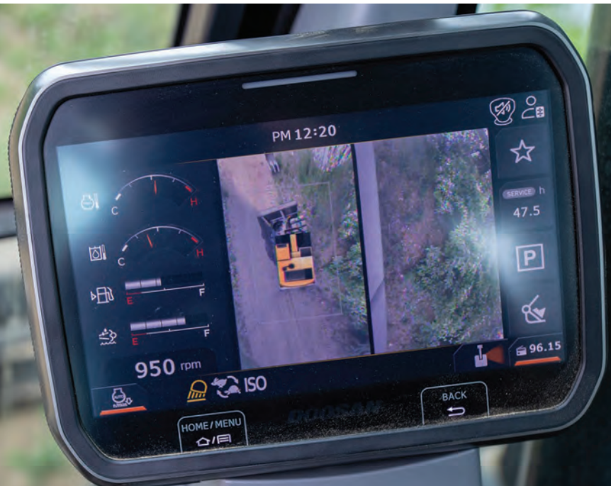
Machine: E145 8-Inch Display With 360 All-Around View Monitoring Camera
