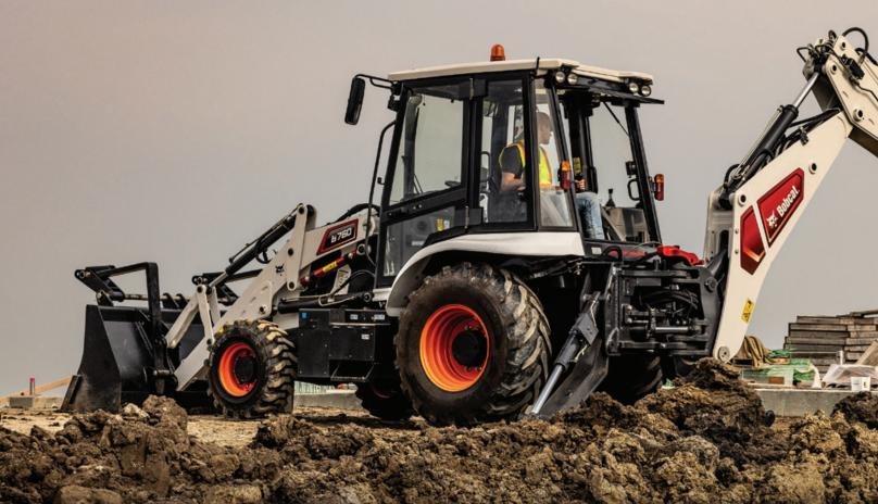
The Bobcat® B760 is an outstanding center-pivot backhoe loader that's designed with durability, easy operation, simple maintenance and incredible performance in mind. This digging, trenching and loading workhorse delivers 96 horsepower and nearly 180 degrees of backhoe swing for the job – without sacrificing essential maneuverability and jobsite accessibility.
